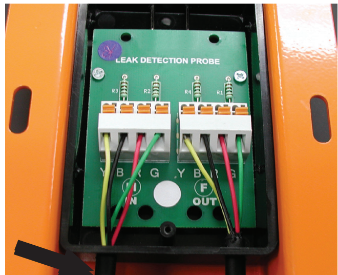
Figure 3. Multiple probe wiring configuration and suggested tie wrap location
